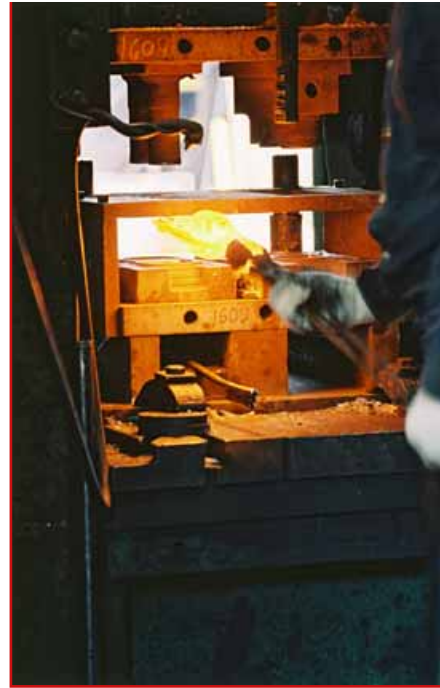
Anchor Forgings being Trimmed & Pierced in 150 Ton Minster Trim Press
