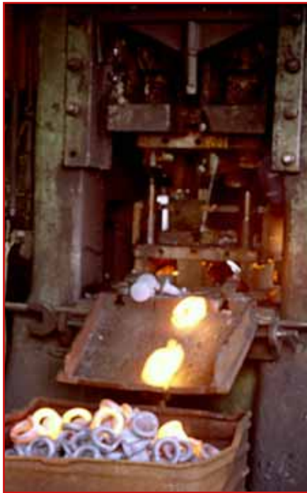
Trimmed & Pierced Anchor Forging dropping into material handling container
