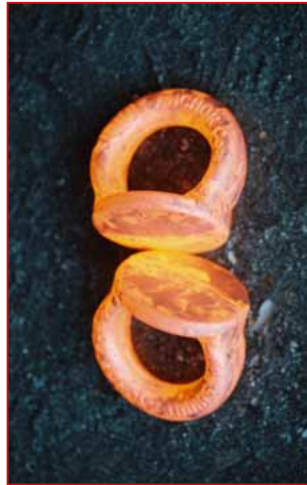
Close-up View of Trimmed & Pierced Anchor Forging
