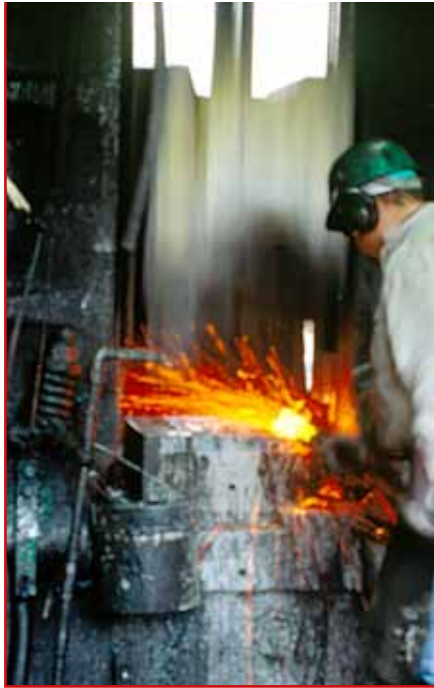
Anchor Forgings being manufactured in a 2,500 lb Double Acting Erie Forge Hammer
