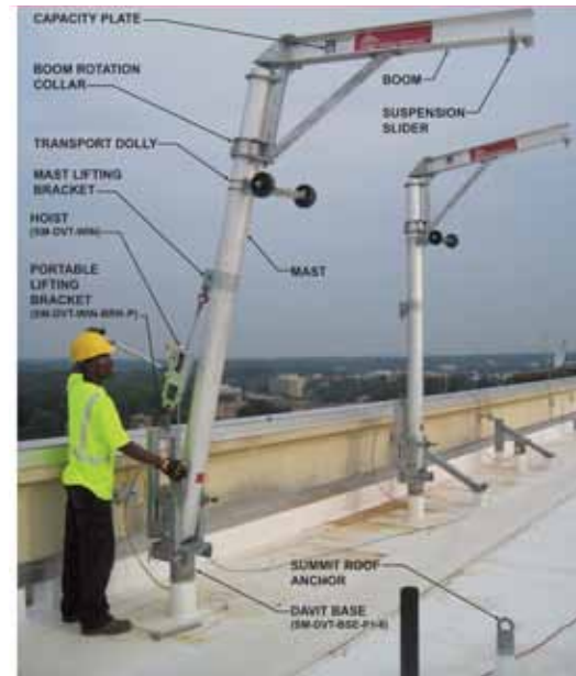
SM-DVT-ARM-TR-x-** Davit Arm - Top Rotating -* Specify either 6 ft. or 8' Boom Reach -** Specify either 1,250 lb. or 1,000 lb. Capacity
