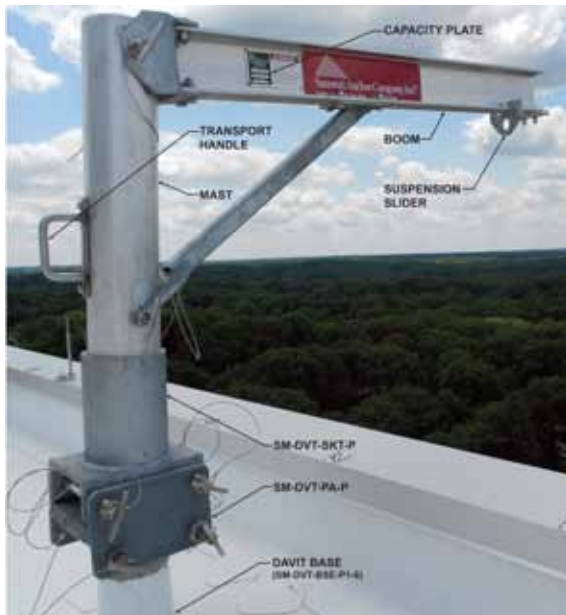
SM-DVT-ARM-x-** Davit Arm - Ground Launched -* Specify either 6 ft. or 8' Boom Reach -** Specify either 1,250 lb. or 1,000 lb. Capacity
