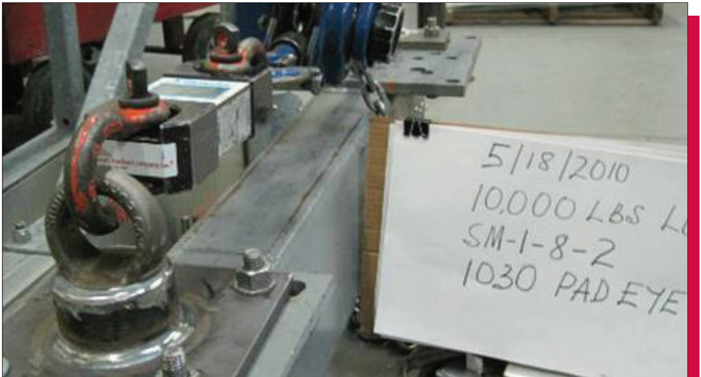
Fig. 5. Testing Summit's Forged Eye to 10,000 lbs.
