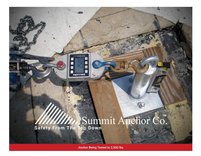
Both OSHA and ANSI-I.14 require two independent anchorages for each worker attached. Anchorage layout requirements are more fully addressed in an anchor layout guide for rope descent systems. Anchor Layout Manual
