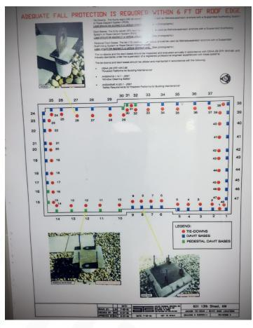
Above anchorages rigged by Rope Descent Workers in horizontal direction, whereas the roof door plan posted on the inside of the roof door said: "load should be applied in the vertical direction only.
