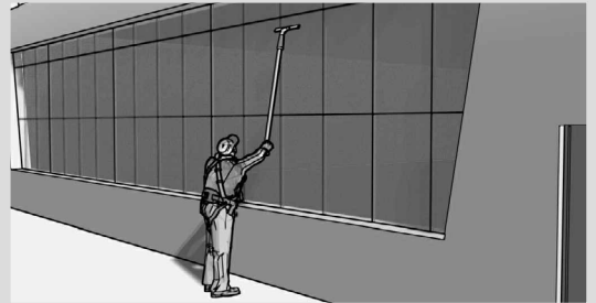
DOING WORK AT GROUND LEVEL RATHER THAN IN HEIGHTS, IF POSSIBLE
